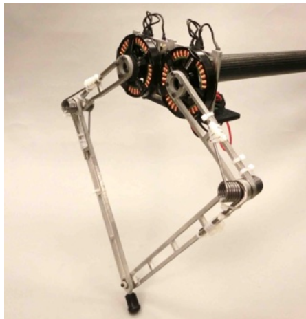
Figure 2.7: Closed Kinematic Chain Leg using Raibert's Scissor Algorithm (Duperret, Koditschek, 2016).[3]
